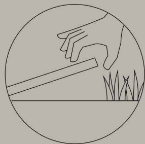
Posa su erba/ Dry laying on grass
